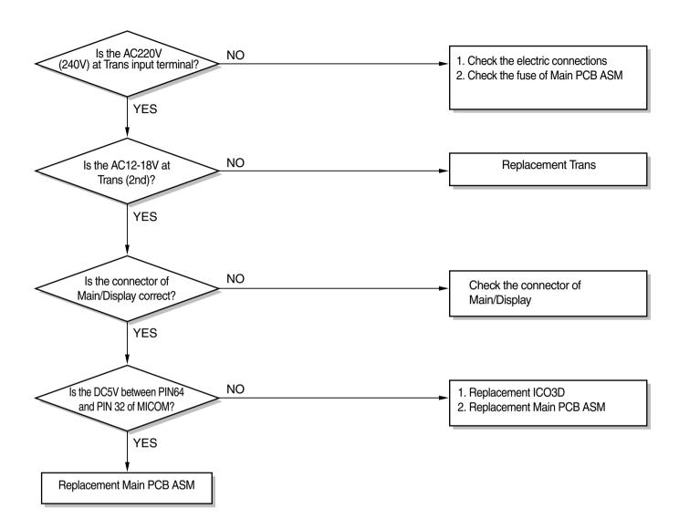
6) Timer control does not operate. Replacement Micom
